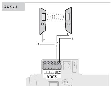
A connected photocell is automatically detected by the controller as soon as the power supply is connected. The photocell can be retrospectively reprogrammed.
